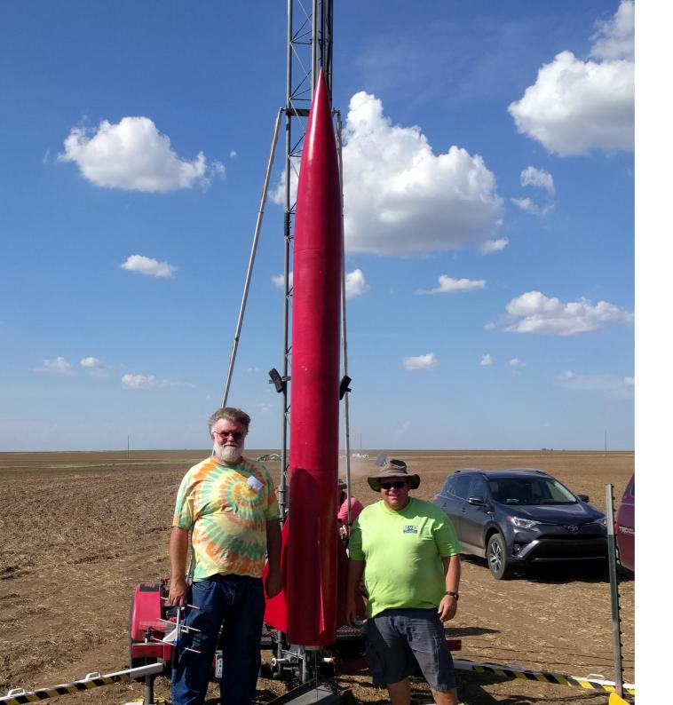
"O"-class motor 76kg at launch 3km+ apogee!
